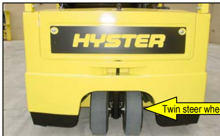
Hyster steering actuator and twin steer tires
