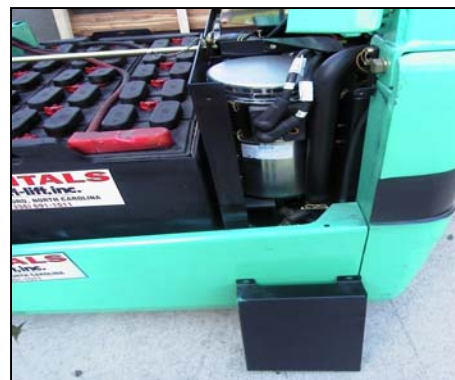
Mitsubishi power steering and hoist motor access with floor plates removed
