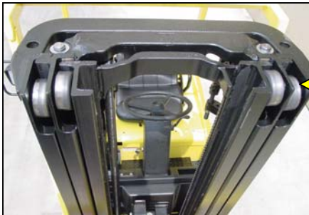
Canted load roller design
