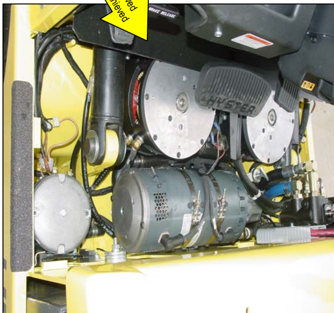
Hyster power steering and hoist motor access with floor plates removed
