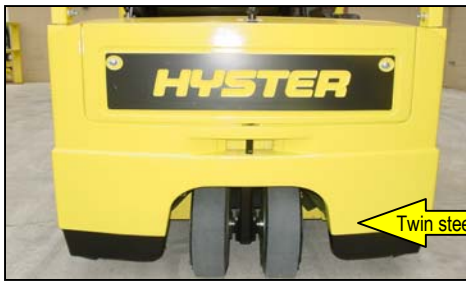
Hyster twin steer tires and steering actuator
