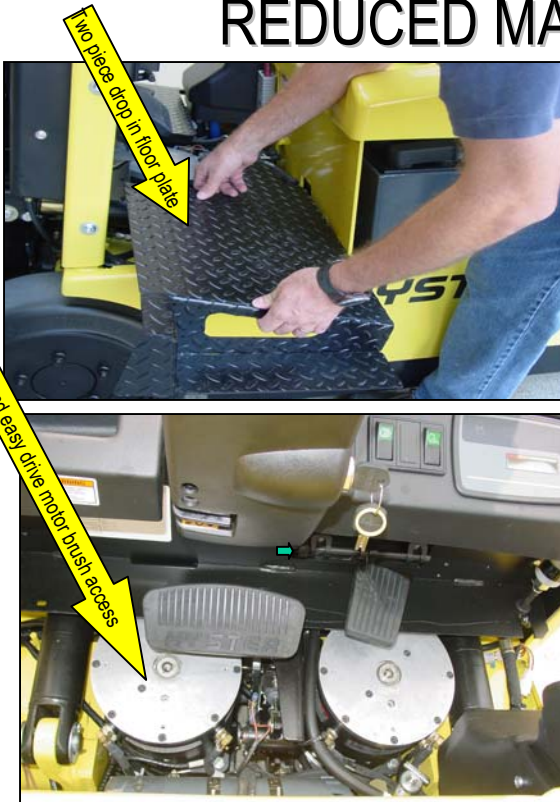
Hyster drop in floor plates and Drive motor brush access
