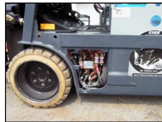
Toyota Electrical system (floor plate already removed and not shown in above picture)
