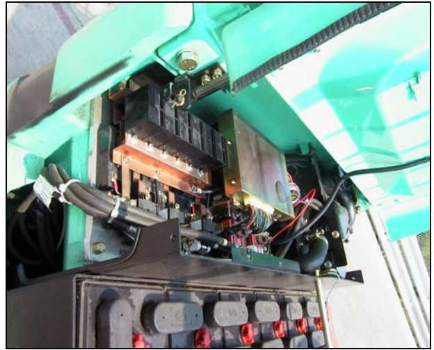
Mitsubishi TR4000 SX Transistor Controller
