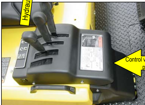
Hyster hydraulic control board and connecting linkages
