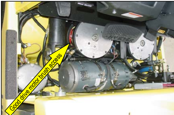
Hyster drop in floor plates and drive unit motor brush access
