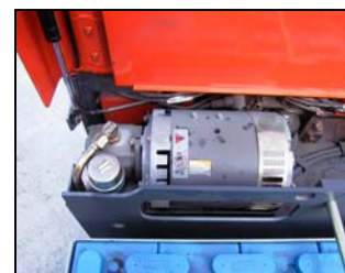
Toyota power steering and hoist motor access (floor plates not shown)
