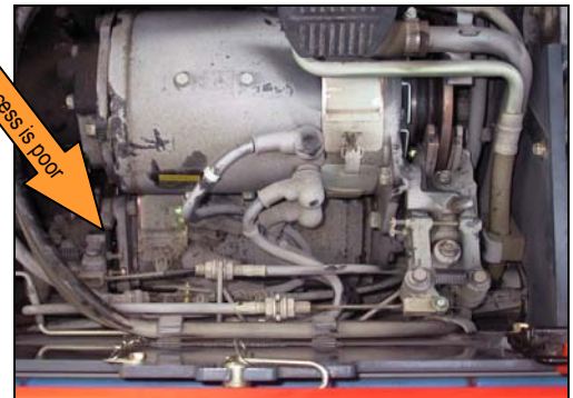
Toyota Power Cables and Brake Discs
