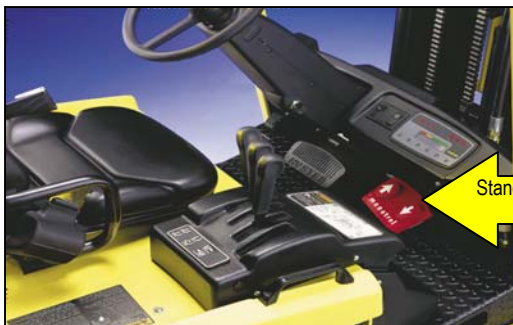
Hyster floorboard area layout and standard accelerator pedal options
