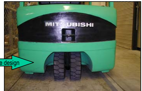
Mitsubishi twin steer tires and steer actuator
