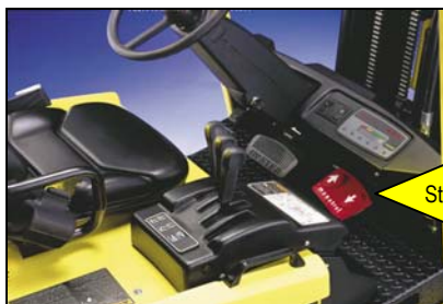
Hyster floorboard area layout and standard accelerator pedal options
