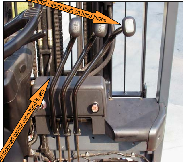
Toyota Control Valve Handles
