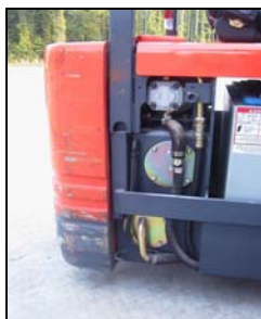
Toyota power steering and hoist motor access (floor plates not shown)
