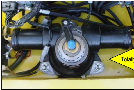
Open gear mesh Enclosed hydrostatic steer actuator
