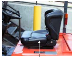
Wing back type seat has no hip restraints, therefore, provides no grab point for entering or exiting the operator's compartment.
