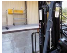
Hard plastic hand grip (RH Side Only) located 58" from floor.
