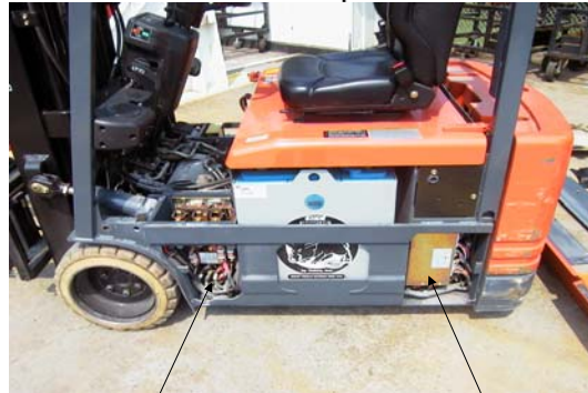
Contactor panel assembly includes: line, hoist, steer and directional contactors
