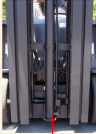
Crown cylinder has less protection
