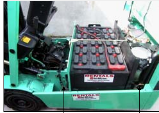
Main hydraulic supply line routed from front to back
