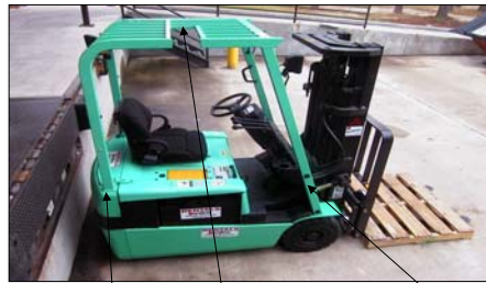
Counterweight mounted overhead guard; rear legs
