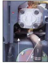
Hydraulic pump & motor is shock mounted
