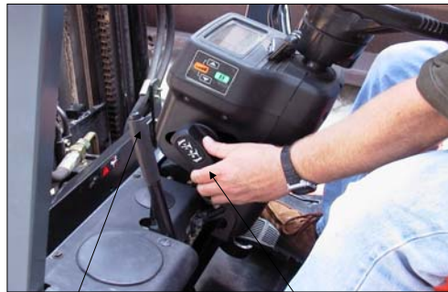
Hand applied and released parking brake
