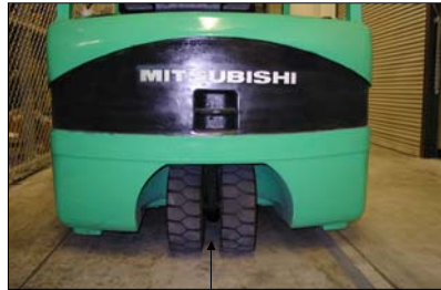
Hydrostatic steer system with twin steer wheel design
