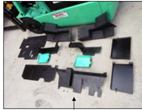
Service access panels and covers. There are 12 total access panels and covers, 21 bolts and screws. Requires 3 different type wrenches and a Phillips screw driver.
