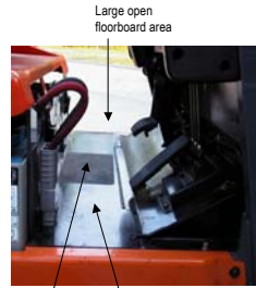
8" X 12" Skid Pad Metal floor plates with no tread or substantial skid pad for entering and exiting the operator's compartment.
