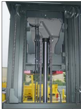
Two 6 conductor over the mast wire cables
