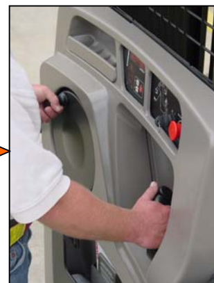
Raymond multifunction control handle and operator console
