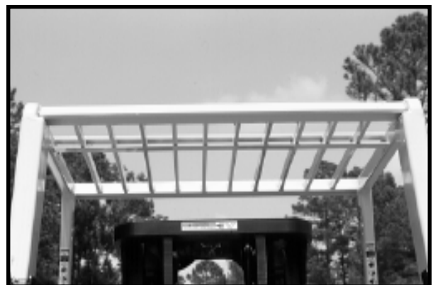
Interlaced steel bar on edge overhead guard
