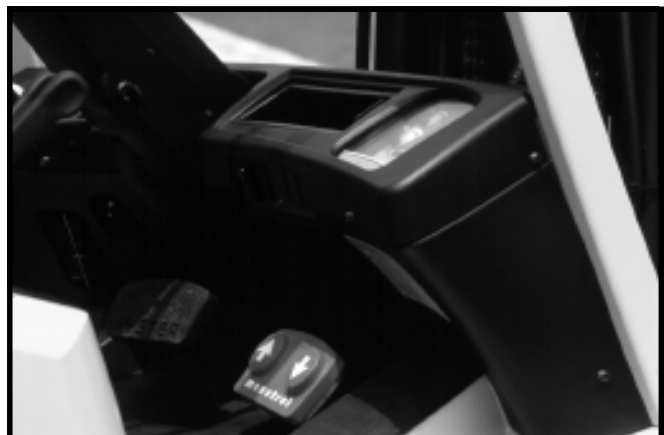
Monotrol provided as standard equipment
