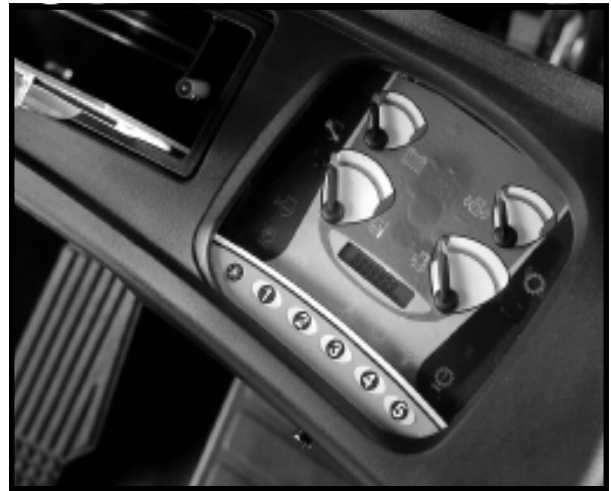
Engine shut-down system controlled through instrument module
