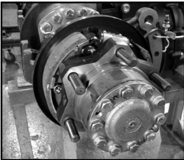
Outboard mounted drum brakes
