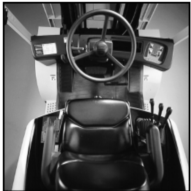
Adjustable steering wheel and column
