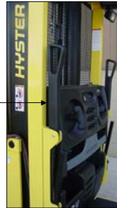
View of side gates in fully retracted position
