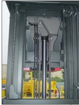
Two 6 conductor over the mast wire cables
