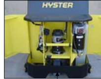
Service compartment with access doors open
