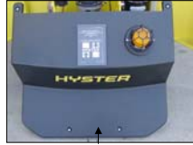
ABS plastic rear cover with mounting hardware
