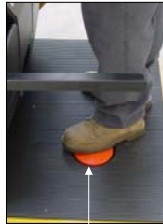
Ergonomically positioned foot switch
