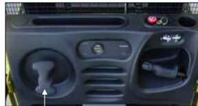
Standard RTC (Return To Center) steering
