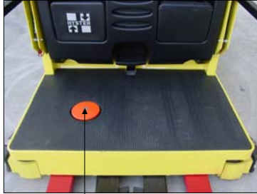
Flush mounted electric foot switch
