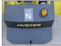
ABS plastic rear cover with mounting hardware
