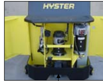
Service compartment with access doors open
