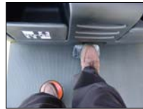
View of operator activating the foot switch and pallet clamp release pedal
