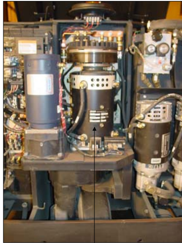
Master Drive unit (MDU) assembly
