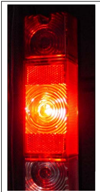
Existing Brake and Backup Light package with incandescent bulbs
