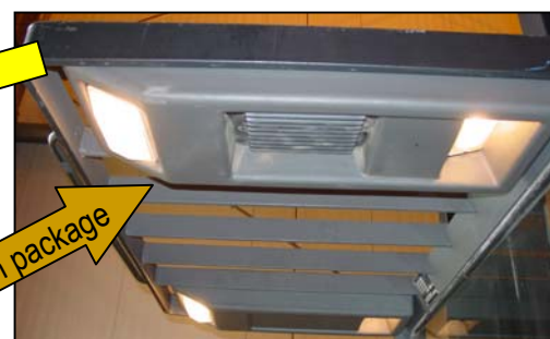
Crown operator compartment cover and light and fan package
