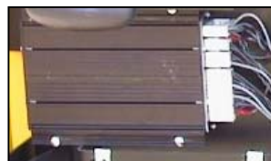
Hyster traction motor and MCU (Master Control Unit)
