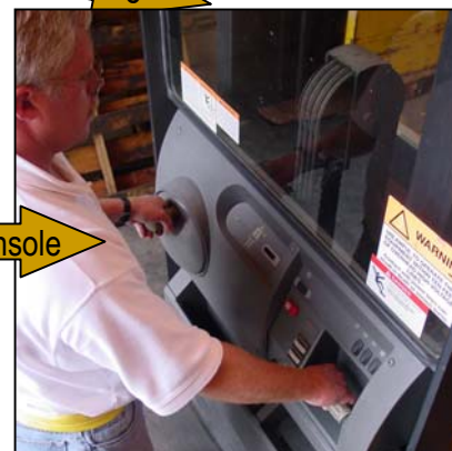
Crown accelerator handle. Crown does not offer an adjustable console
