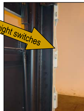
Crown accelerator switch and Crown height sensing switches
