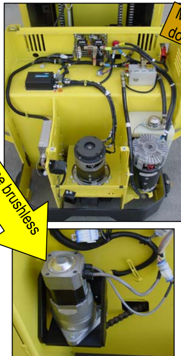
Hyster motor compartment access and brushless power steering motor
